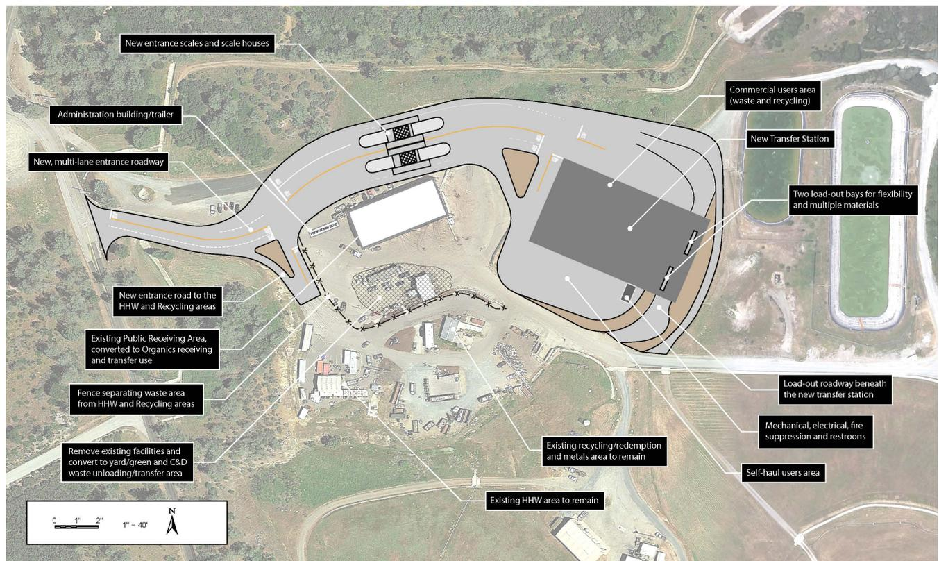
**Figure 4 Transfer Station Plan**
